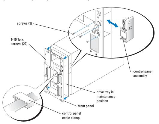
Figure 1-6. Removing/Installing the Control Panel Assembly and Front Panel
