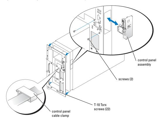
Figure 1-17. Removing the Rack Control Panel Assembly
